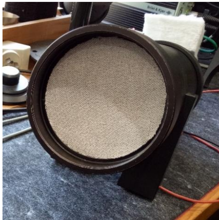
Figure 1 Phonic & Audible samples installed in large tube
